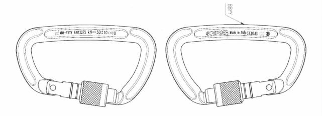
Placement of the marking: Partially printed and partially engraved on the body of the connector.
